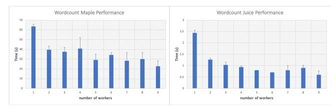
As we can observe, as the number of workers increases, there is a decreasing trend in the time used to finish both maple phase and juice phase. Using 9 workers (the maximum number of workers) can improve the performance of one single worker by 64% during maple phase, and 75% during juice phase. The comparison between the performance of Hadoop and MapleJuice is shown in the following graph.
